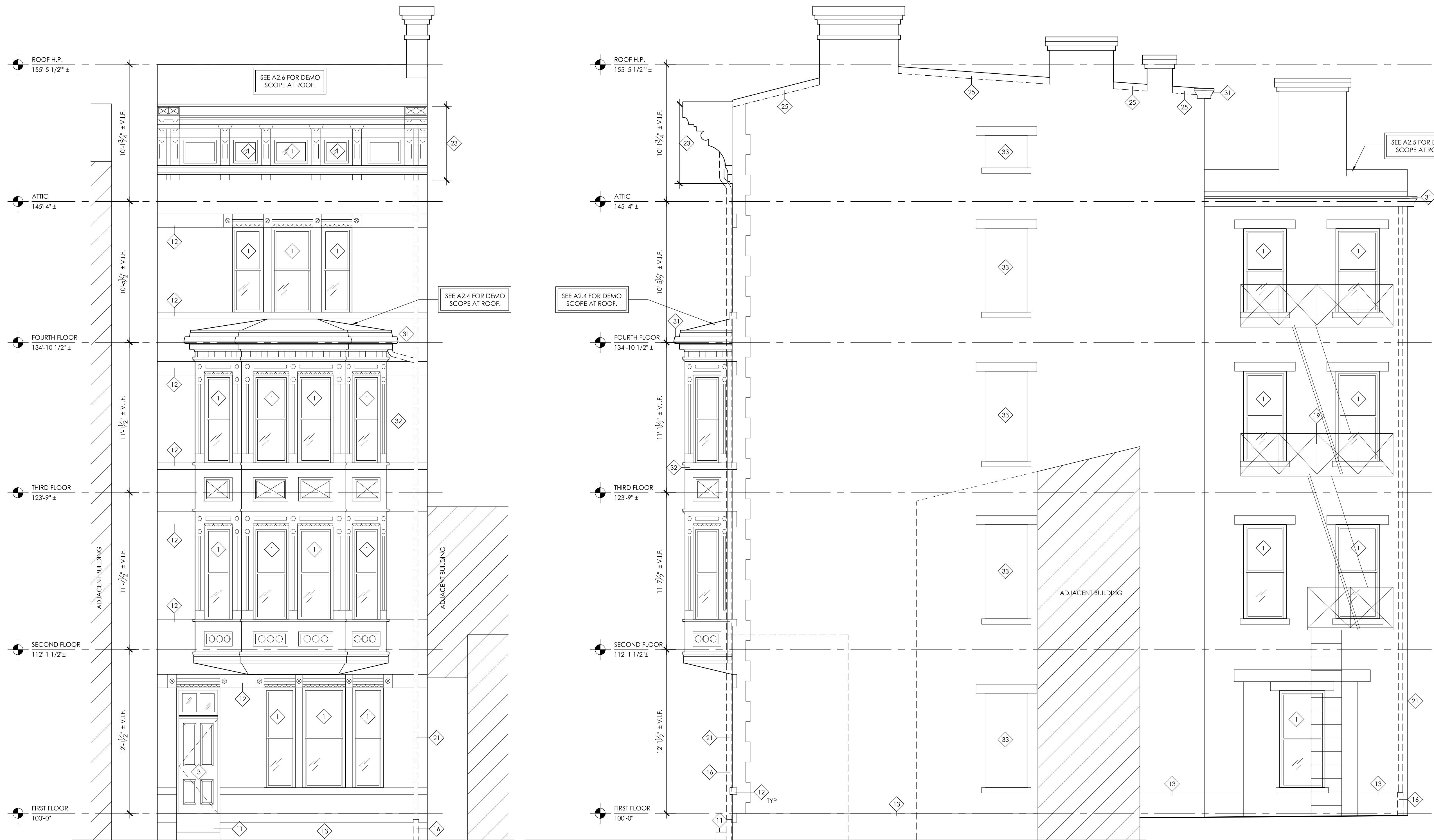
1 SOUTH DEMOLITION ELEVATION
