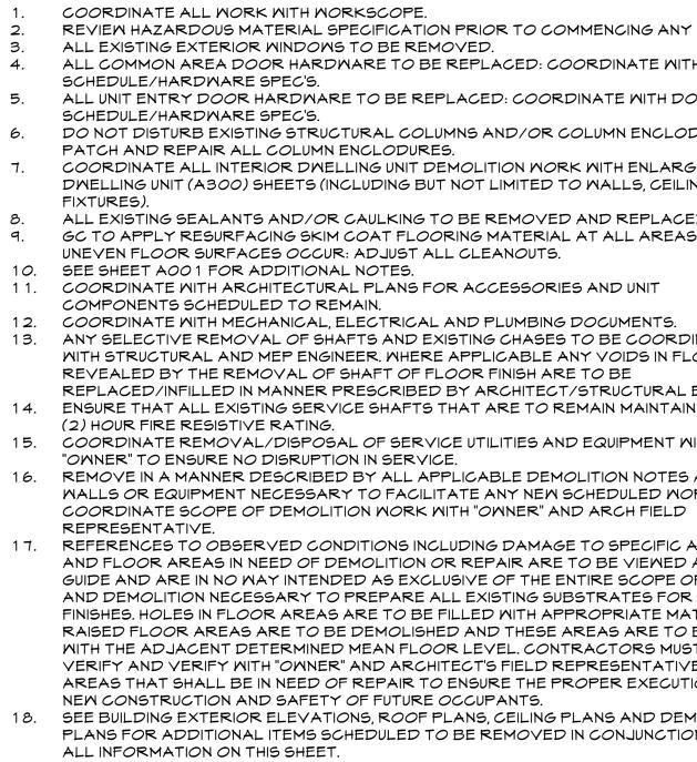
REVIEW HAZARDOUS MATERIAL SPECIFICATION PRIOR TO COMMENCING ANY WORK. ALL COMMON AREA DOOR HARDWARE TO BE REPLACED: COORDINATE WITH DOOR ALL UNIT ENTRY DOOR HARDWARE TO BE REPLACED: COORDINATE WITH DOOR
