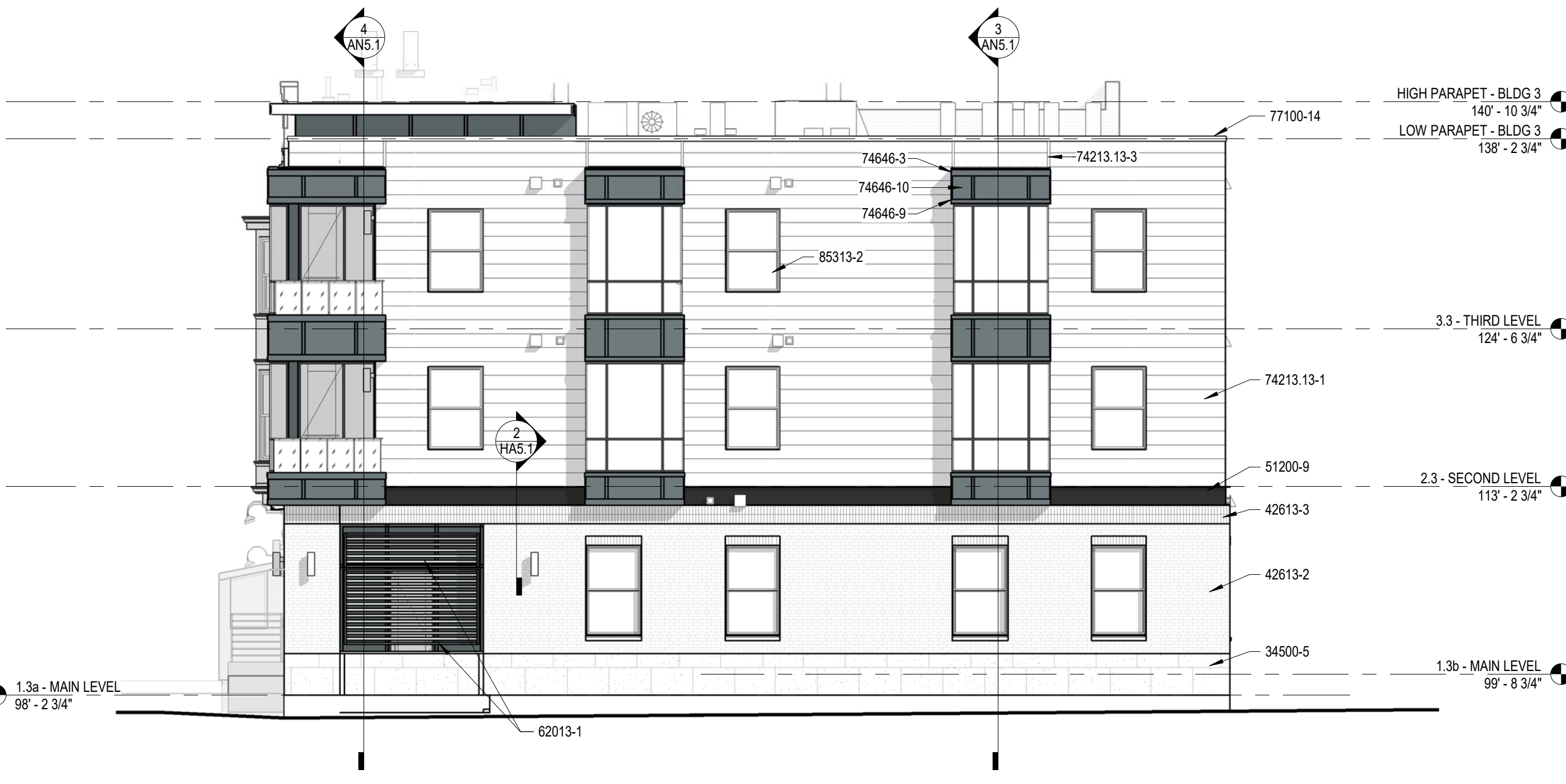
1 EXTERIOR ELEVATION - SOUTH - NEW BUILDING 3 SCALE: 1/8" = 1'-0"
