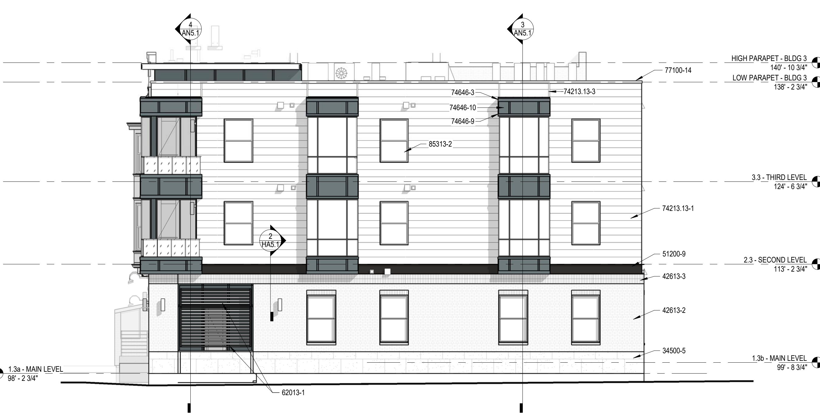
1 EXTERIOR ELEVATION - SOUTH - NEW BUILDING 3 SCALE: 1/8" = 1'-0"
