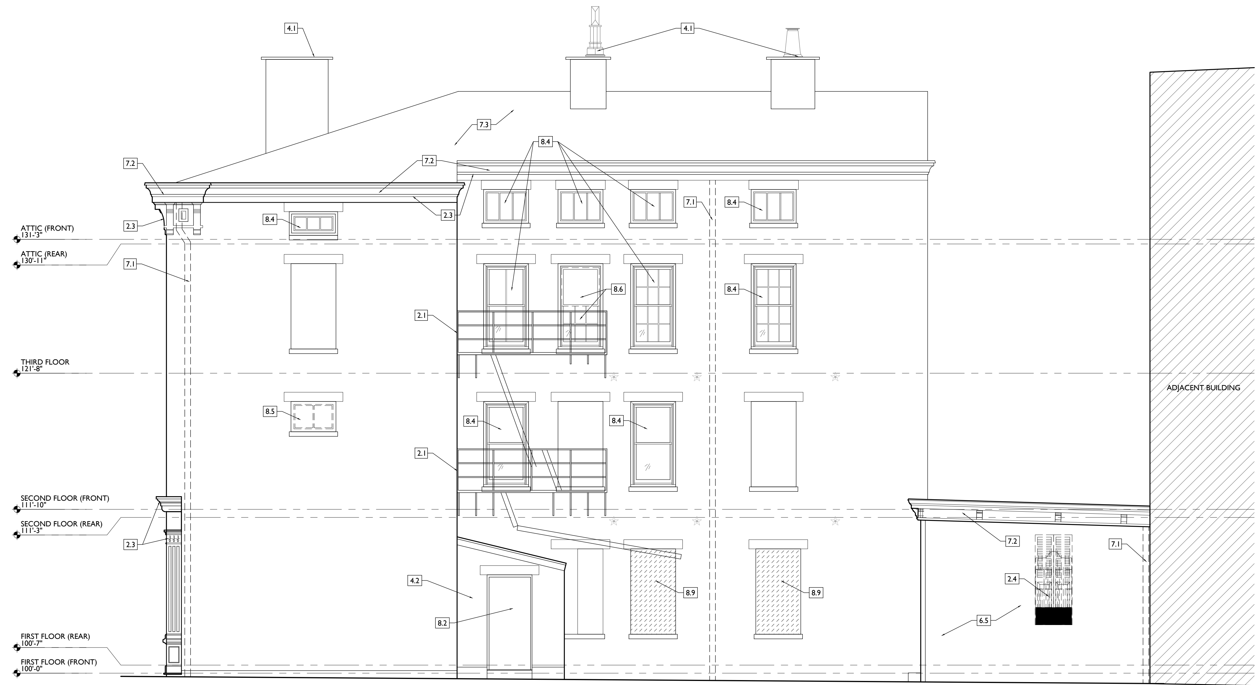
SCALE: 1/4" = 1'-0" EXISTING + DEMOLITION ELEVATION - NORTH | 1
