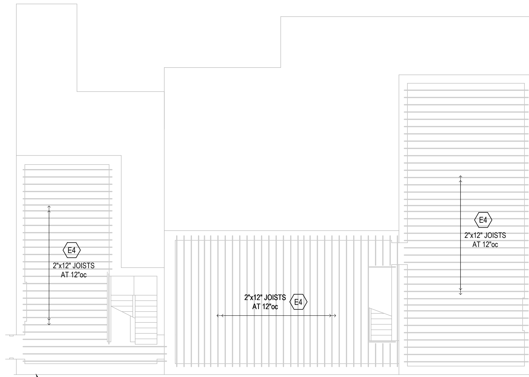
SECTION 3 - FIRST FLOOR FRAMING PLAN
