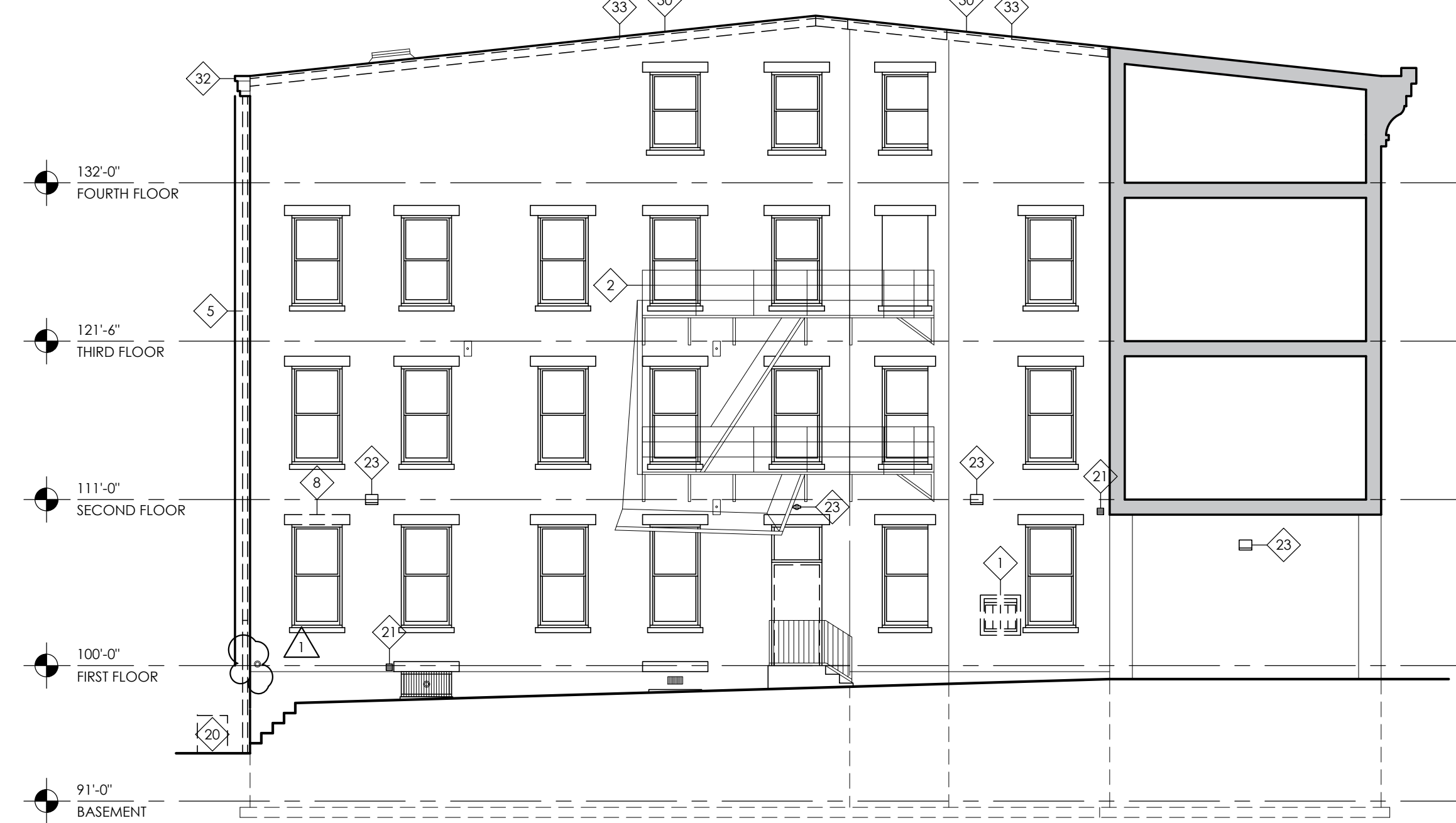
2 EAST DEMO ELEVATION A4.0 1/8" = 1'-0"
