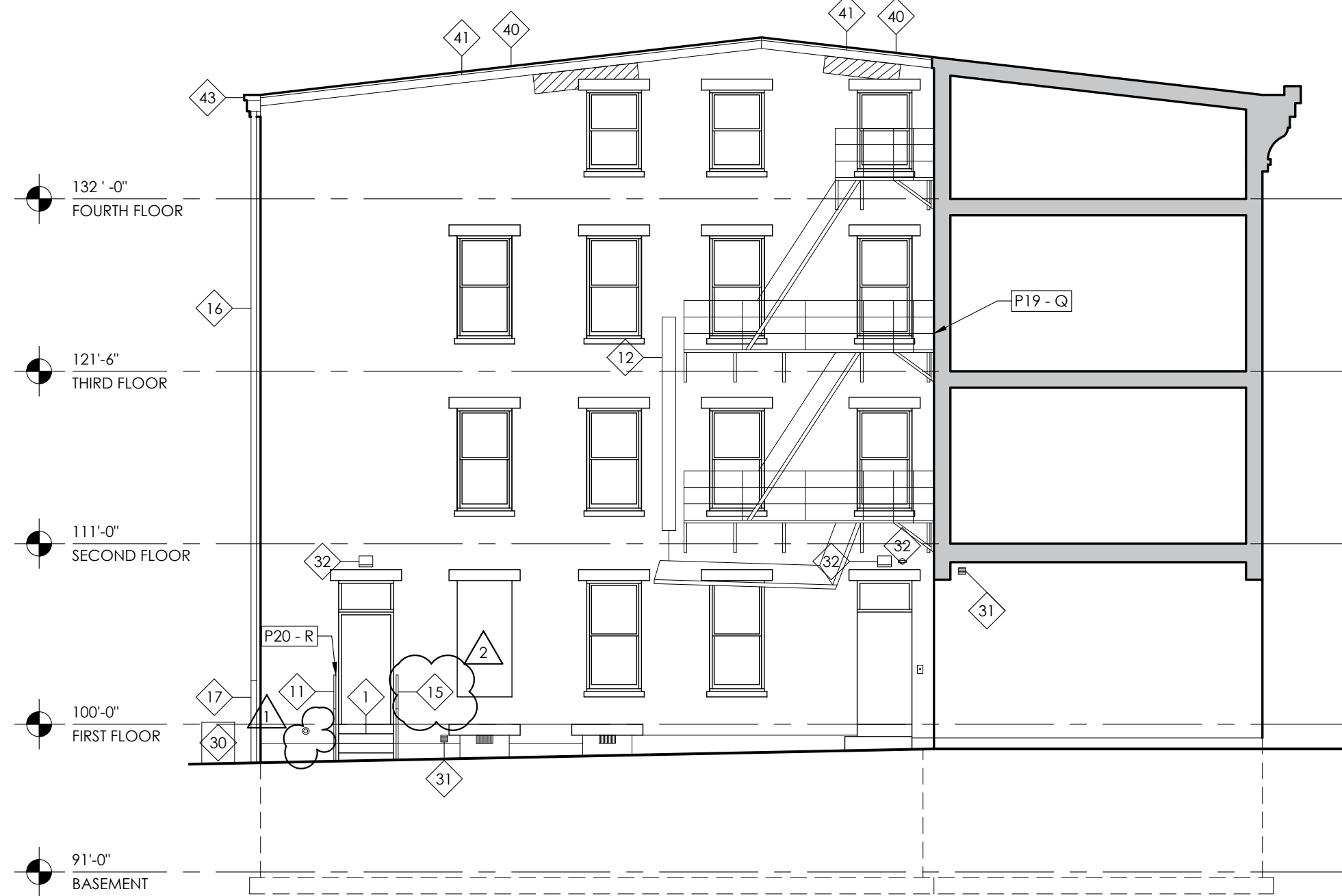
2 EAST NEW WORK ELEVATION A5.0 1/8" = 1'-0"
