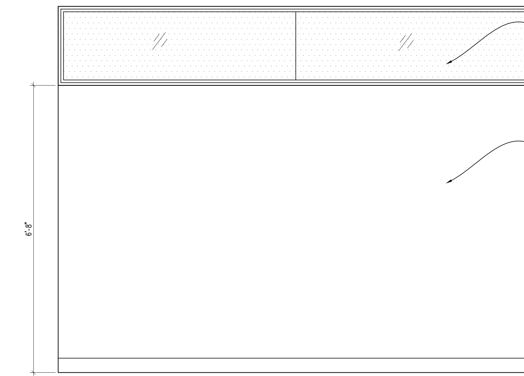
GLASS TRANSOM WALL ELEVATION SCALE: 3/4" = 1'-0"
