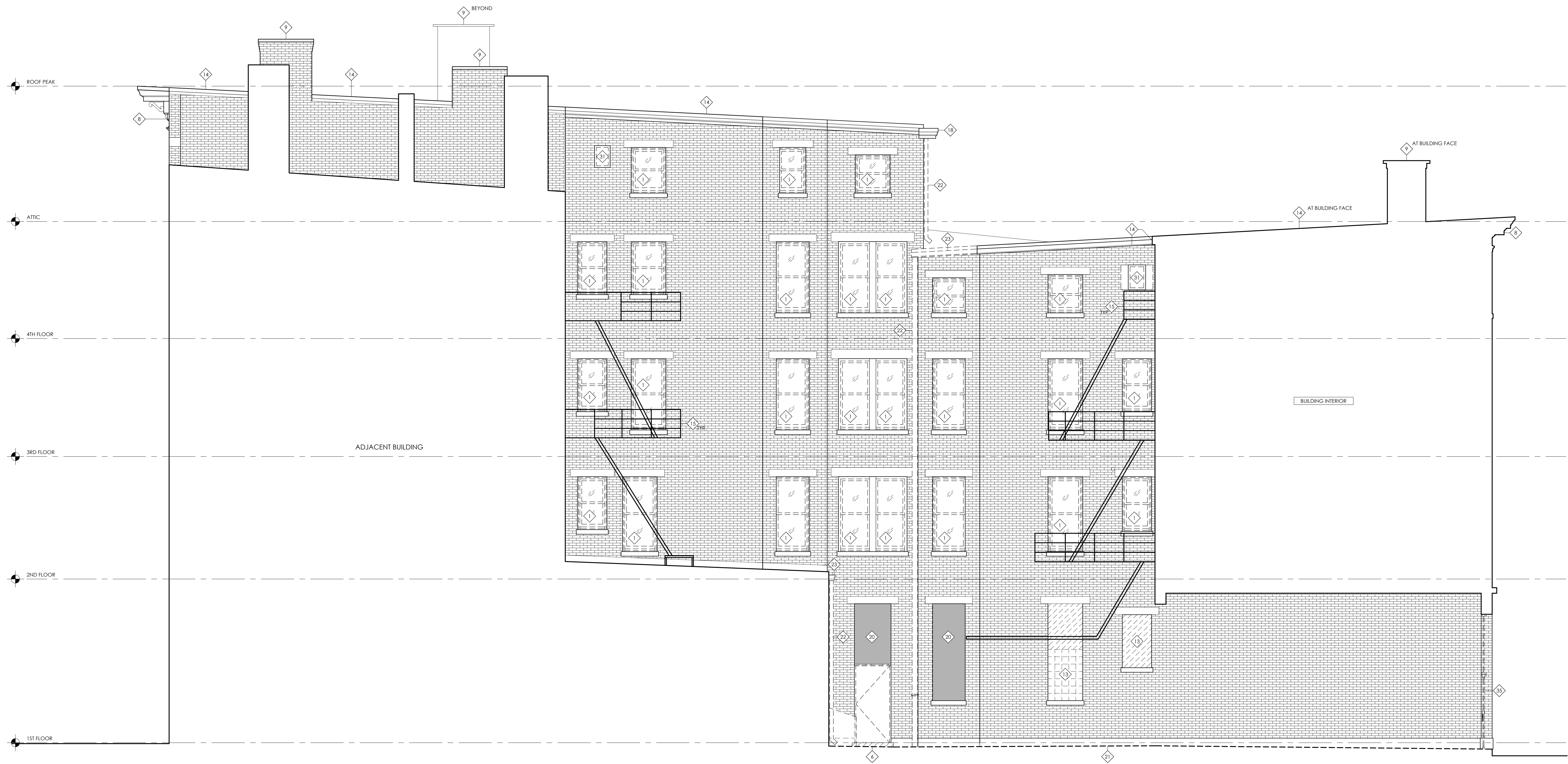
1 A5.3 1/4" = 1'-0" DEMOLITION NORTH EXTERIOR ELEVATION
