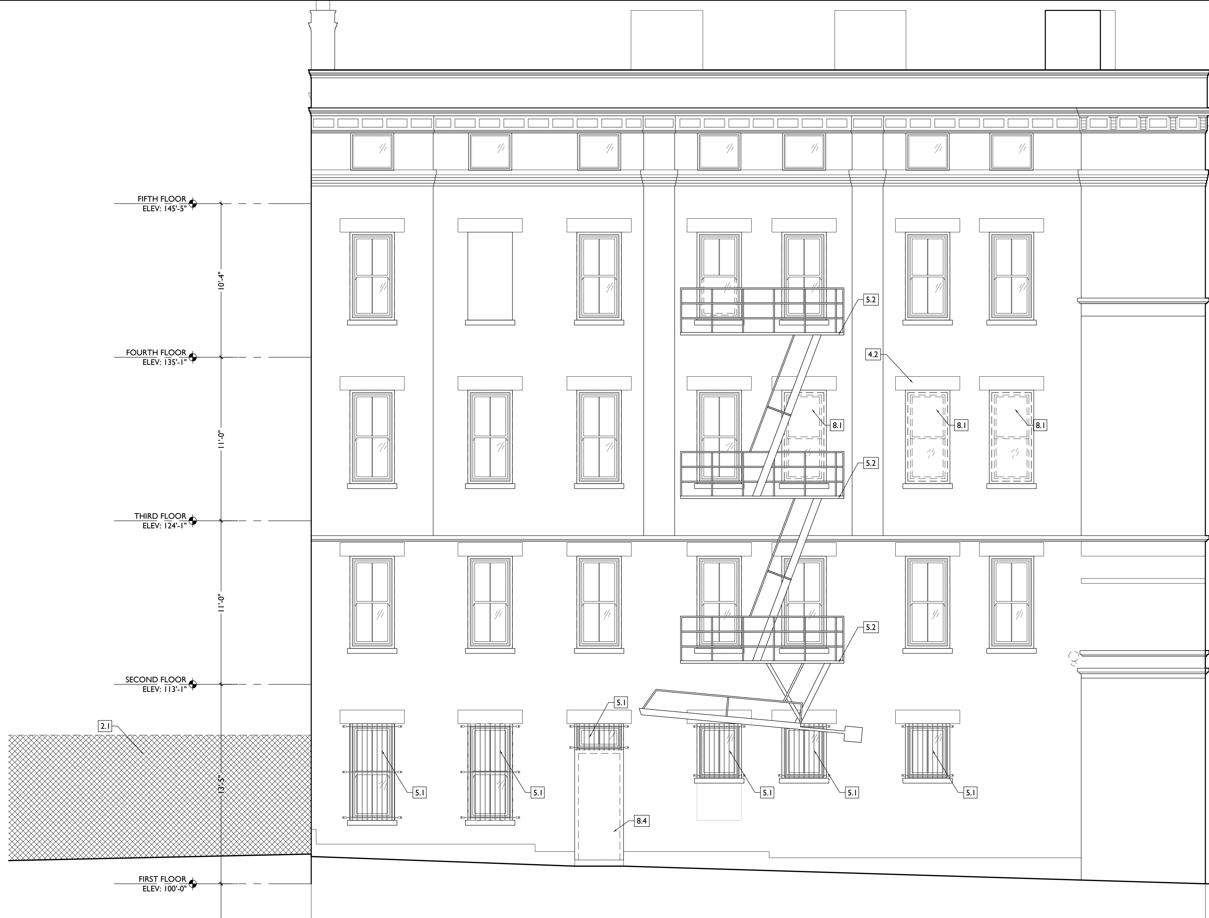
SCALE: 1/4" = 1'-0" EXISTING + DEMOLITION ELEVATION - NORTH |
